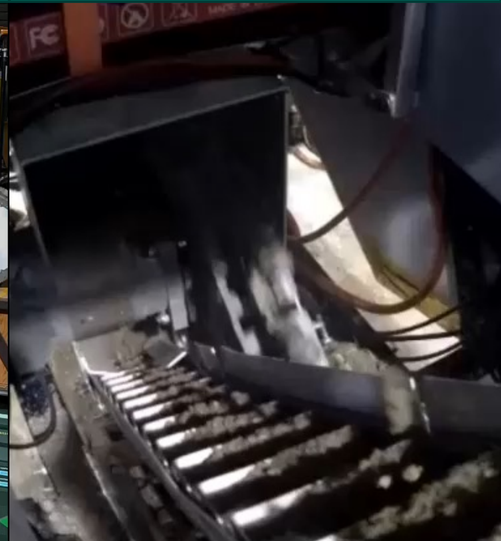
Conveyor chain failure
